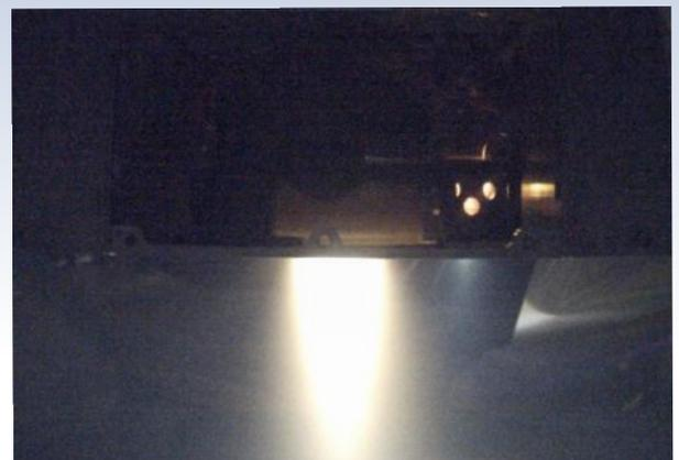
**BIT-3 RF Ion with Iodine Propellant**
